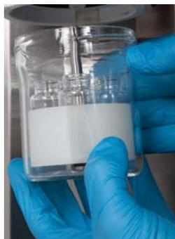
*miVac SpeedTrap is supplied with a one litre glass condensing vessel.*
